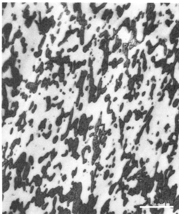
Figure 2. Transmission electron micrograph of a thin section prepared by ultramicrotomy of an undeformed bulk specimen of PS/SEBS-LM at 25 wt % block copolymer.
